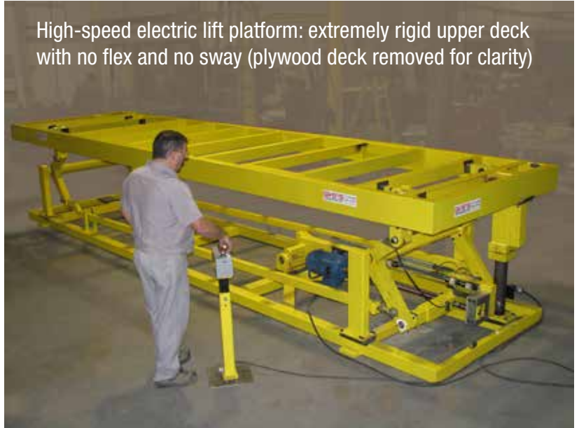
Hydraulic tandem lift platforms for auto assembly line workers
