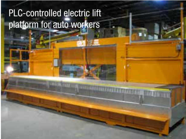
Hydraulic scissor lift for extracting car bodies from the assembly line for testing
