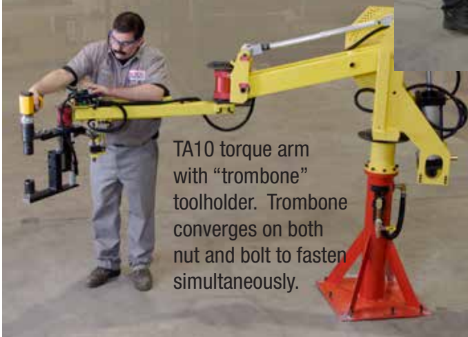
Trombone close-up, incorporates rotation
