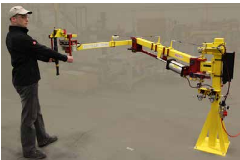
▲ TA5 torque arm with complex, braked toolholder. Nutrunner can rock left and right from vertical to access screws on a slant.
