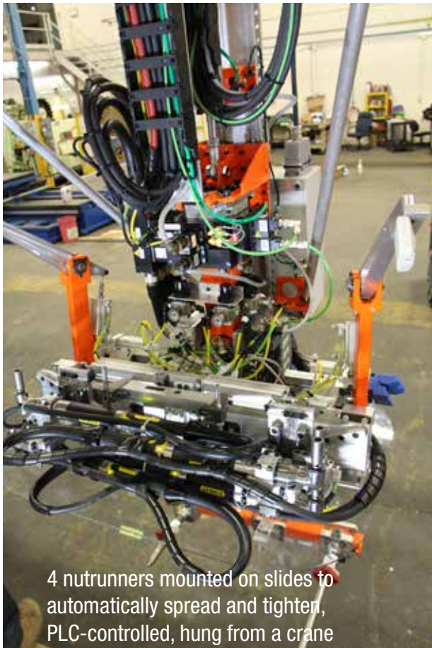
Givens manipulator with hatch and nutrunners
