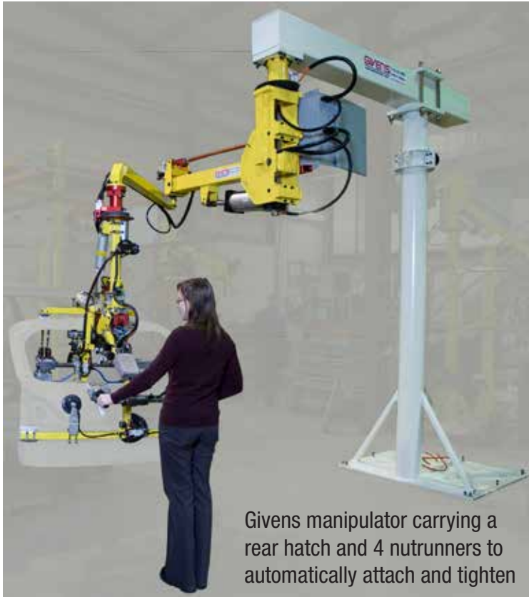
Tooling holding 4 nutrunners passing through the hatch opening
